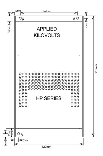
Fixing Holes 3 off M4 Clearance holes marked 'A'
